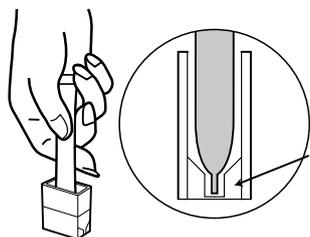
insert the PACKTEST in the groove, as shown.
