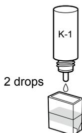
(1) Fill the Cell (PACKTEST Square Cup) up to the first line (1.5 ml) with sample. Add 2 drops (~0.07mL) of K-1 reagent.
