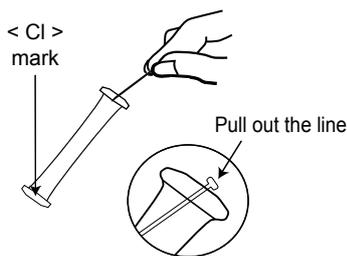
(3) Remove the line to clear the aperture from the top of the tube.
